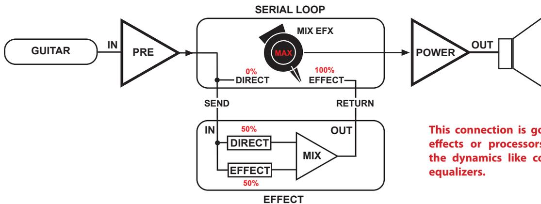
This connection is good for stomp effects or processors that act on the dynamics like compressors or equalizers.
