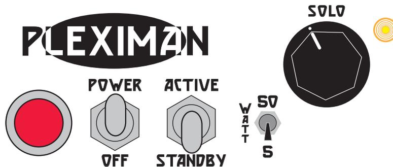
The Pleximan also has a 'SOLO' function as seen on the Customwork series. This convenient function more than doubles the output volume of the amp and is controlled via a simple footswitch.
